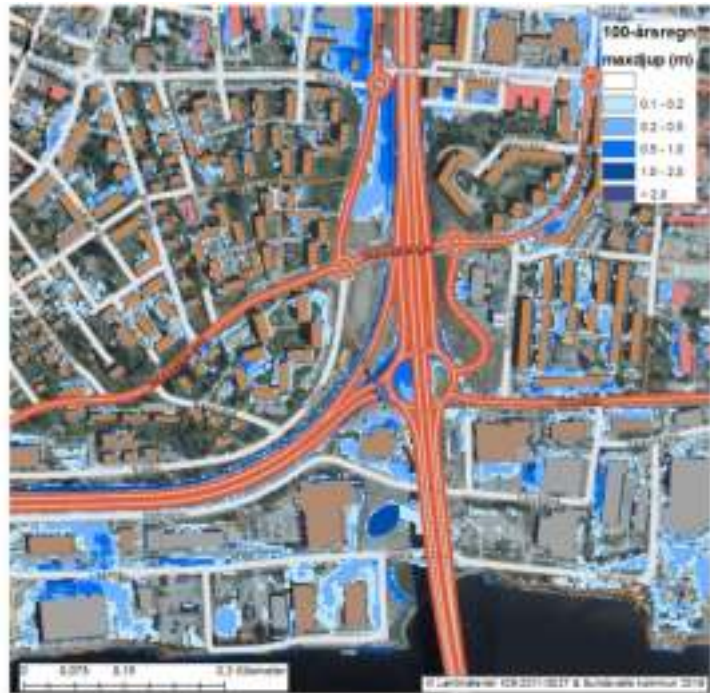
Image 12. The E4 at the northern abutment in a simulated 100-year rainfall event.
