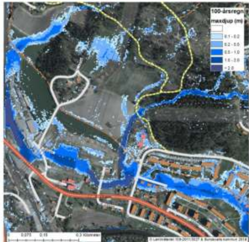
Image 10. Granlo Electrical Substation in a simulated 100-year rainfall event.
